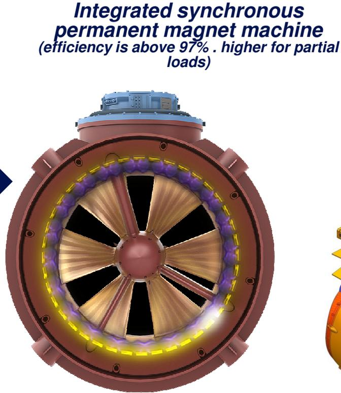
**Integrated synchronous permanent magnet machine**
