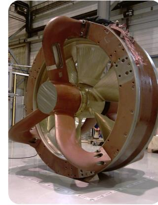
Assembly of 1<sup>st</sup> commercial PMTT1600, 800kW
