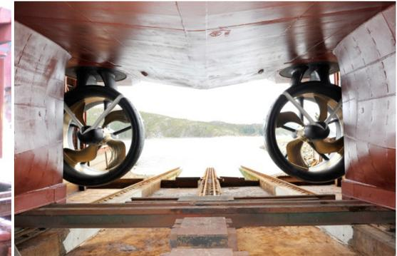
**Propulsion system : 2x500kW, 440V 60Hz
