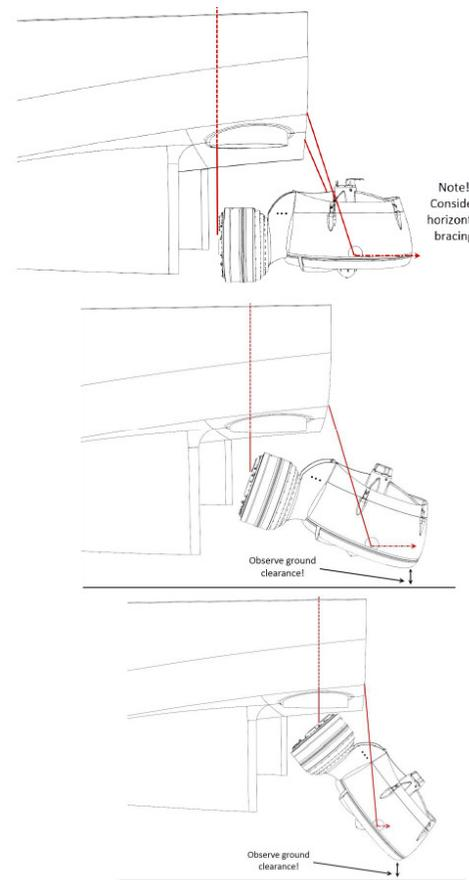
Figure 3.2-9 Lifting and up-ending thruster
